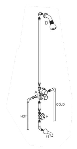
Water Harmony thermostatic valve with ¾" ceramic disk volume control
