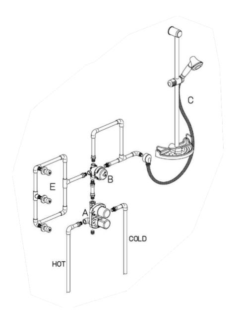
Ornellaia thermostatic valve with ¾" ceramic disk volume control
