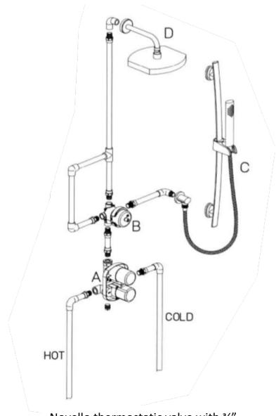
Novello thermostatic valve with 3/4" ceramic disk volume control 8" rain shower head with 12" arm Slide bar kit 3-way diverter Rough included.
