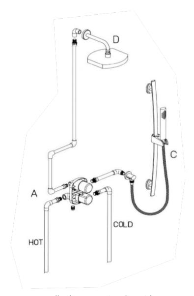
Novello thermostatic valve with 2way diverter volume control 8" rain shower head with 12" arm Slide bar kit Rough included.
