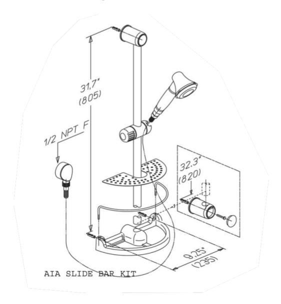
Ornellaia 30" slide bar kit Includes: Hand shower, wall mount bracket and supply elbow, 78" flexible hose
