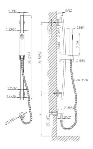
Lady 30" slide bar kit Includes: Handshower, wall mount bracket and supply elbow, 78" flexible hose
