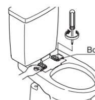
**5** Remove Template. Align Washlet in front of Base Plate. Slide Washlet onto Base Plate until there is a click.
