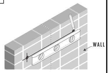
3 Once position is marked, drill 2 holes and insert anchors if stud is not available
