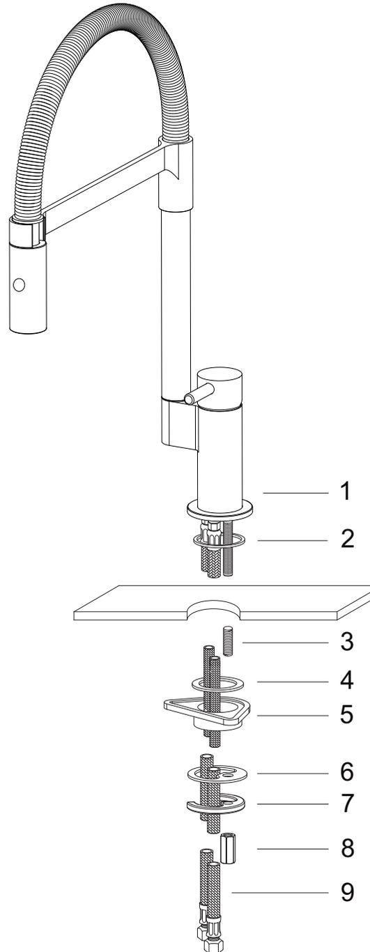
6. Cut a mounting hole 1 3/8 diameter (35mm) in the desired position in counter top or sink (if one isn't available).
