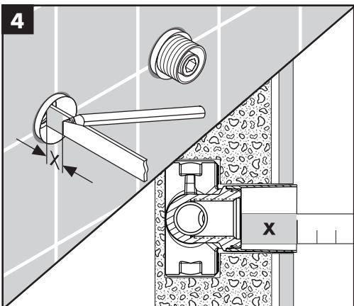
Measure the distance from the spout outlet of the rough to the outside of the plaster shield ("X").
