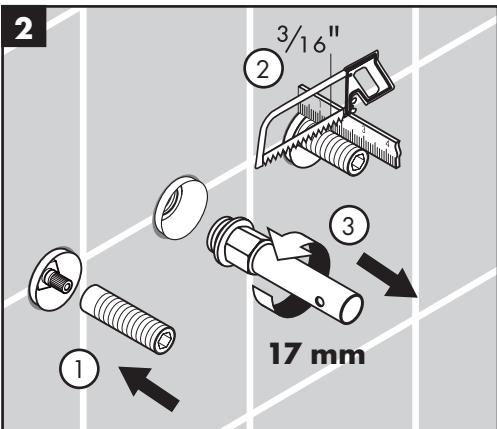
Install the spindle extensions.
