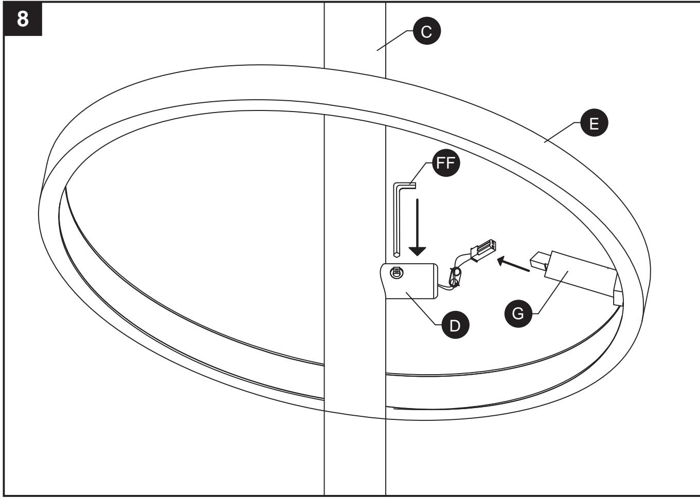
8. Raise small LED ring (E) to fixture body (C). Connect wiring from arm (D) to swivel (G). Insert swivel (G) into arm (D) and secure with set screw using the allen tool (DD). Repeat this step for medium LED ring (H), large LED ring (F), and extra-large LED ring (L).
