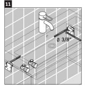
Using the appropriate bit for the wall material, drill pilot holes.
