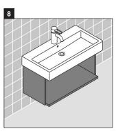
Slide the vanity under the washbasin. Tighten mounting bolts with a wrench until the washbasin is stable.
