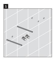
Reference the washbasin specification and furniture specification (page 1) to establish the height and spacing of the mounting bolts.
