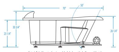
Note: Infinity 2 is not a drop in model.  $\,$  A deck must be built around the tub.
