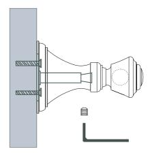
Using the Allen Key provided, loosen the Bar Posts' Set Screws.
