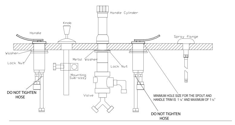
\*\*\* NOTE: SHUT OFF WATER SUPPLY BEFORE BEGINNING INSTALLATION\*\*\*
