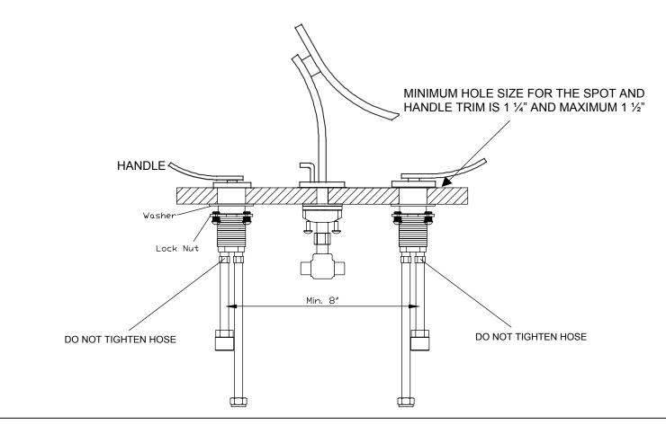
\*\*\* NOTE: SHUT OFF WATER SUPPLY BEFORE BEGINNING INSTALLATION\*\*\*
