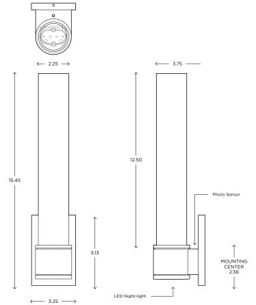
This fixture mounts independently from diffuser/backplate. The outlet box is located behind the diffuser.
