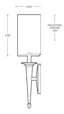
This fixture mounts independently from diffuser/backplate. The outlet box is located behind the diffuser
