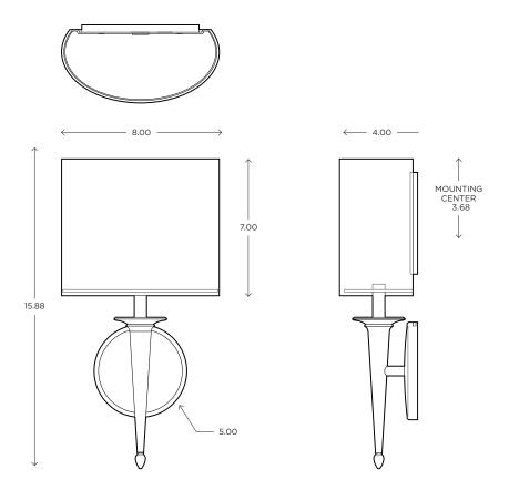
This fixture mounts independently from diffuser/backplate. The outlet box is located behind the diffuser
