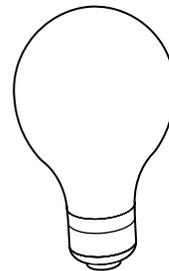
This fixture requires a 100W Max Incandescent lamp to fit its Incandescent Medium Base socket.
