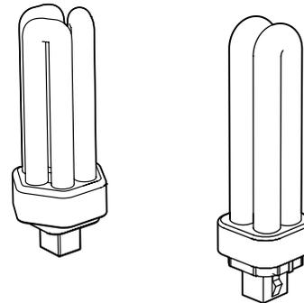
This fixture requires a 18W 4-pin, 2700K or 3000K CFL **Quad or Triple Tube** to fit the fixtures Gx24q-2 socket.
