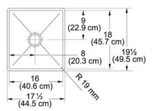
Professional Series sinks are undermounted for an immaculate countertop. If an authentic restaurant kitchen is your fancy, the Professional Series is the real thing. It is designed with sturdy commercial-grade stainless (16-gauge) and is deep enough to accommodate the bulky equipment used by the serious cook.
