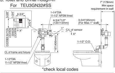
X", ‡ =At least 5" clearance from sensor to tip of toilet seat up position or to top of grab bar is required to aviod false detection.
