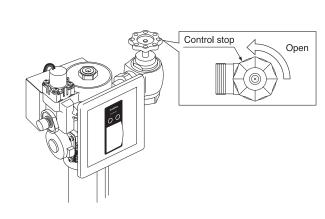
To set the flush valve for proper operation, open the control stop completely and flush several times.
