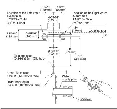
X, ‡ =At least 5" clearance from sensor to tip of toilet seat up position or to top of grab bar is required to aviod false detection. For toilet installation
