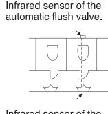
Infrared sensor of the another automatic flush valve.
