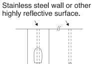
Infrared sensor of the automatic flush valve.
