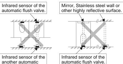
Infrared sensor of the automatic flush valve.
