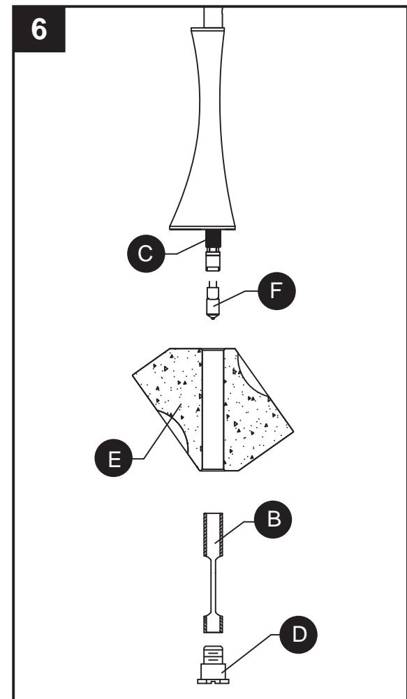
Note: Never touch a halogen light bulb with your bare skin, even when removing the bulb from the package before installing. The oils on your skin will drastically shorten the lifespan of the bulb.
