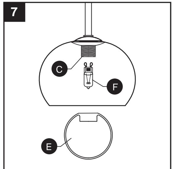
Note: Never touch a halogen light bulb with your bare skin, even when removing the bulb from the package before installing. The oils on your skin will drastically shorten the lifespan of the bulb.
