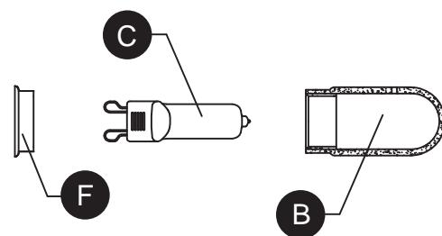
4. Pass shade shade (E) over threaded socket (D) and secure with threaded socket ring (F). Insert 25-watt G9 bulb (C) into threaded socket (D). Screw Bulb cover (B) onto threaded socket (D).
