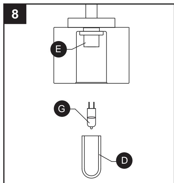
Note: Never touch a halogen light bulb with your bare skin, even when removing the bulb from the package before installing. The oils on your skin will drastically shorten the lifespan of the bulb.
