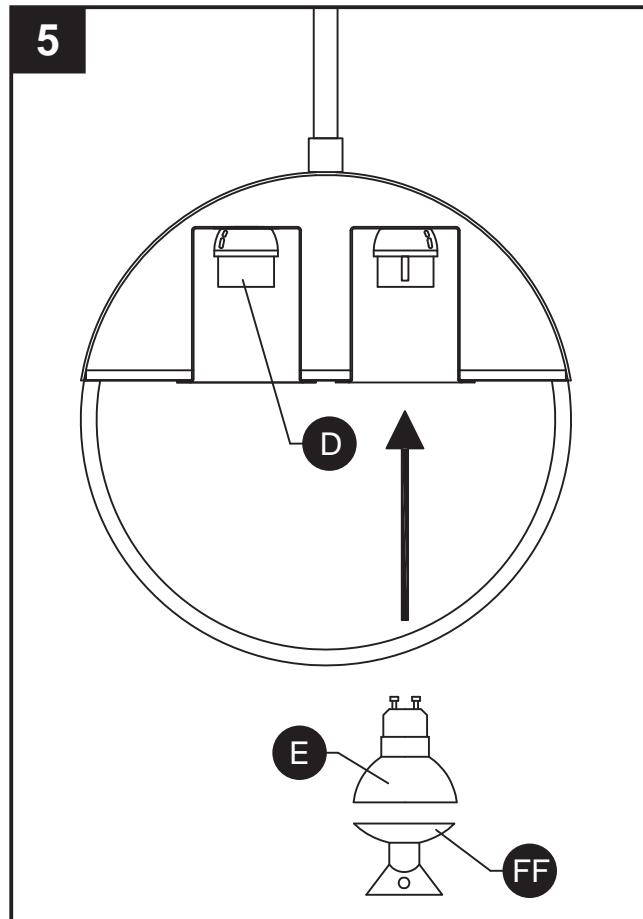
5. Insert two 35-watt GU10 bulbs (E) into socket (D) using spanner (FF).
