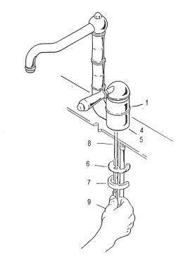
Under the sink, stack the half ring rubber gasket - 6, the half ring mouting plate - 7, then the mounting nut -9 onto the stud.
