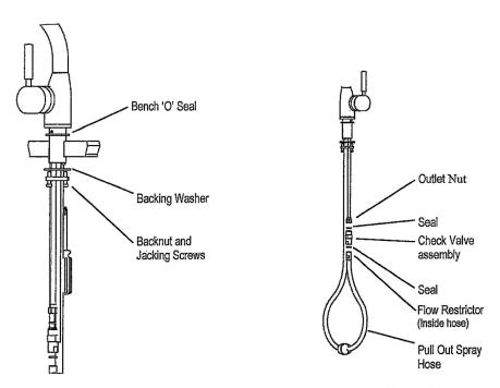
Note: This mixer fits a maximum bench thickness of 2 1/4 inches and has a 140° spout arc.
