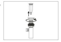
Apply a ring of silicone caulking underneath the drain flange (do not use plumber's putty).
