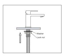
**D** IMPORTANT: After all the connections have been made from inlet supplies to angle stop, remove the aerator. Open the lever on the lavatory. Slowly open angle stop from below and flush the lines for approximately 45 seconds to clean any debris. Turn off the water and reinsert aerator. Debris present in the line will damage fixture and cause leaking. Failure to flush fixture could result in possibly voiding warranty.
