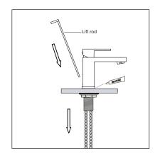
**B** Re-install the washer and lock nut from below.
