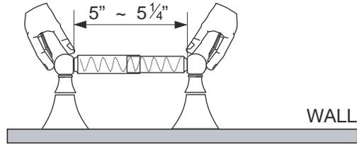
2. Using the mounting hardware position as a reference, mark the screw hole positions in the center of the post flange mark on the wall.
