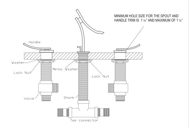
\*\*\* NOTE: SHUT OFF WATER SUPPLY BEFORE BEGINNING INSTALLATION\*\*\*
