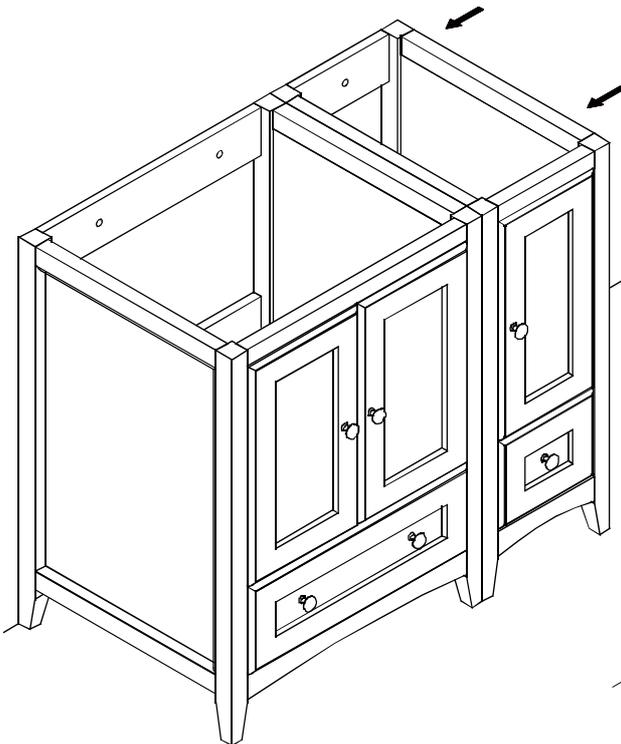
**6** Align and level the rest master cabinet as illustrated shown, then repeat the master cabinet installation procedure.
