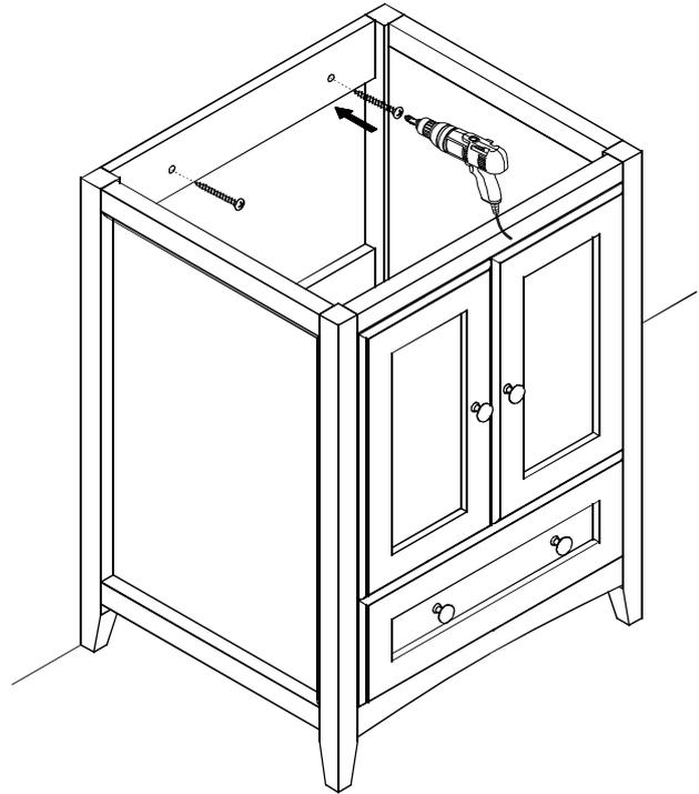
**5** Align and level the side cabinet as illustrated shown, then install side cabinet according to master cabinet installation procedure.
